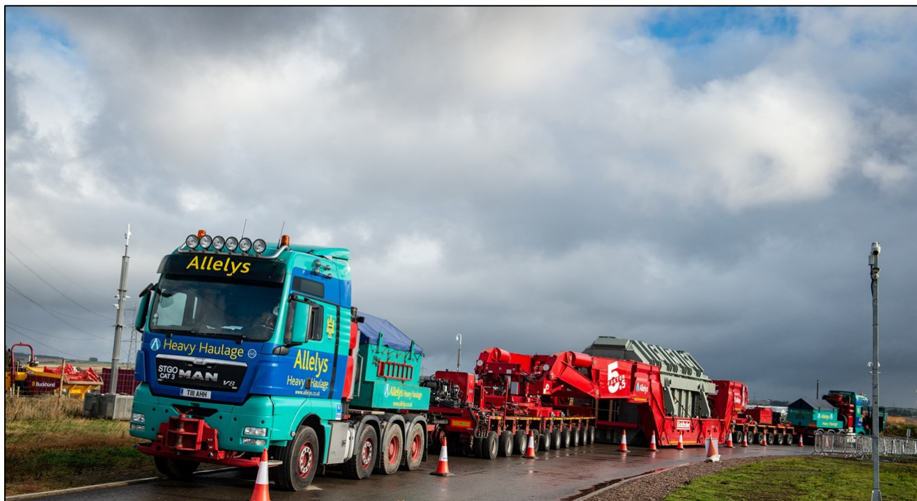
Figure 2-2: Example Transformer Transport
